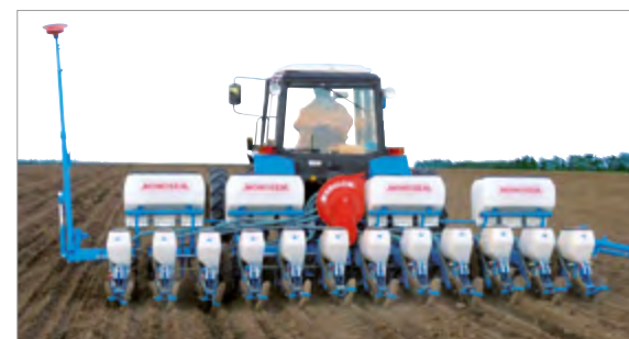
12-row rigid NC Technic Monobar Sugarbeet planter (45cm) – 4x175L fertilizer with tines
